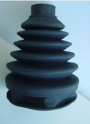
Photo 3, CVJ boot made of ACM//PA TPV.
